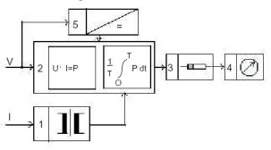
The power converter uses one, two or three for multiplier systems 2 depending on the measurement of balanced or unbalanced load AC systems. Current transformers 1 provide the input current to the multiplier circuit.
